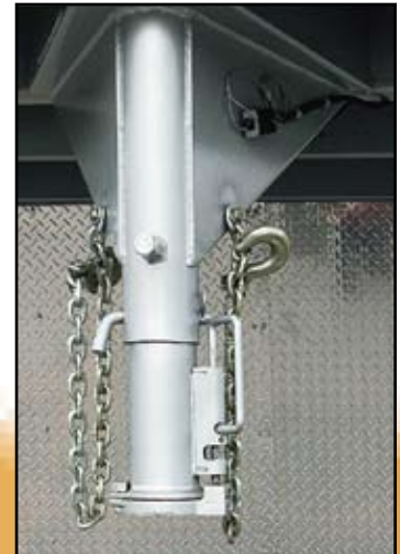
2 5 / 16 Adjustable Height Ball Hitch: Other hitch configurations available as optional equipment.
