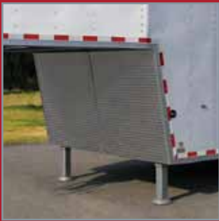
Tandem, 2-Speed Landing Gear
