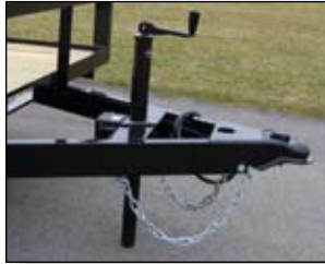
Set-Back Tongue Jack - Clearance for tailgate and SUV rear doors.
