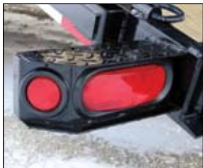
Sealed Recessed Lights - DOT approved lights and reflective tape.
