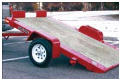
3/4 Decking - Pressure treated plywood 40% stronger than 5/8 plywood.
