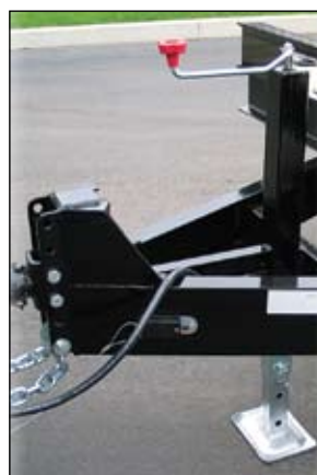
Optional 7000 lb. Drop-Leg-Jack - This rugged design doubles as a spare tire mount.
