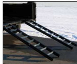
HD Ladder Ramps – Easy access 5 ft. ramps allow for smooth loading/unloading of equipment (Optional on 6 x 10).
