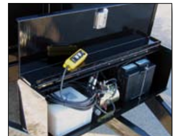
Custom Pump/Battery Box – Lockable Self-latching custom box and long-lasting marine battery. Control Switch operates lift up to 20 ft. away.
