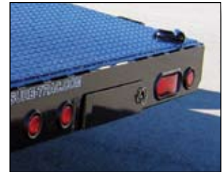
Ramp Compartments – Ramps fit neatly under deck for fast loading and unloading.
